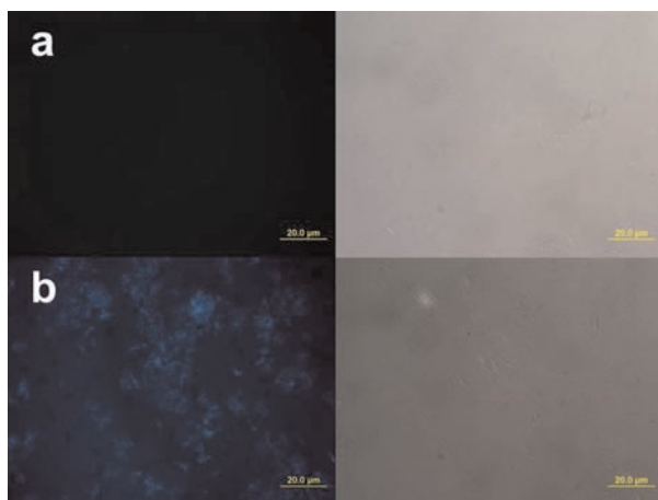
Figure 4. Fluorescence confocal laser scanning images of the ensemble of silole 1 ( 50 \mu\text{M} ), DH ( 0.3 \text{ mM} ) and LOD ( 0.25 \text{ U/mL} ) in the absence (a) and presence (b) of LA ( 0.22 \text{ mM} ). 20
